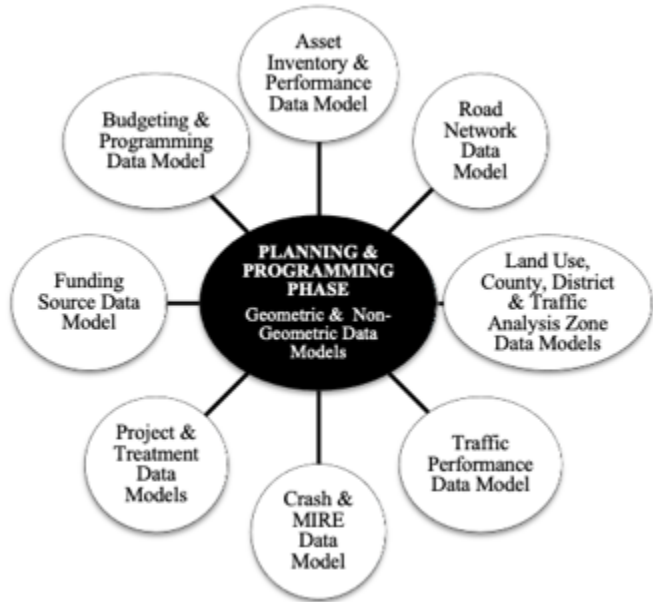
Figure 4. Graphic. Geometric and non-geometric BIM for infrastructure data models used during the planning and programming phase.
