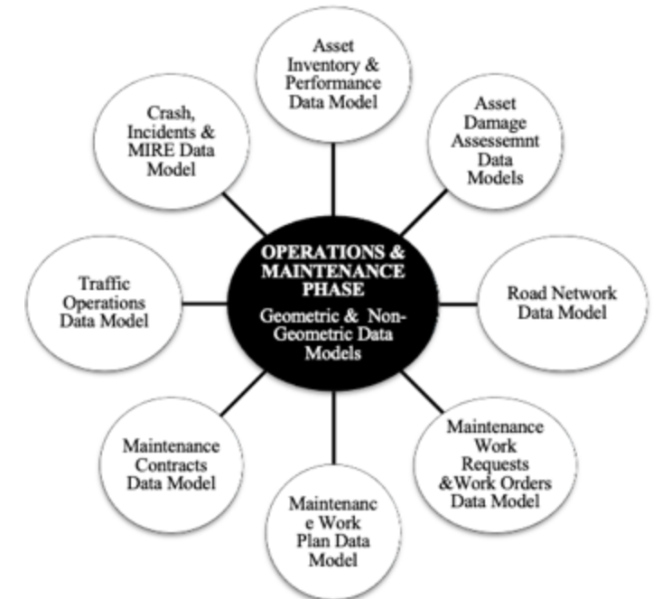
Figure 7. Graphic. Geometric and non-geometric BIM for infrastructure data models used during the O&M phase.
